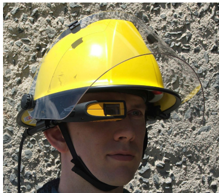
Fig. 4. Head Mounted Display in combination with a helmet [©Liteye Systems, Inc.]
